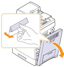
2 Remove the jammed paper, in the direction shown.
